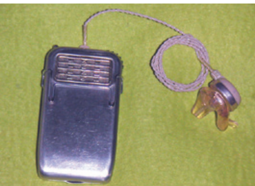
Figure 19. Sonotone's Model 1010 hybrid (1 transistor and 2 vacuum tubes) – the first hearing aid in the world to use a transistor (December 1952).
