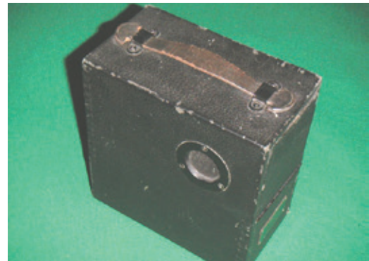
Figure 15. The Globe “Vactuphone” – the first commercially produced vacuum tube hearing aid (1921). This Vactuphone hearing aid still works after all these years. The tube is now 92 years old!
