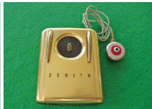
Figure 21. The Zenith "Royal" vacuum-tube hearing aid was one of Zenith's last vacuum tube hearing aids made (February 1952).
