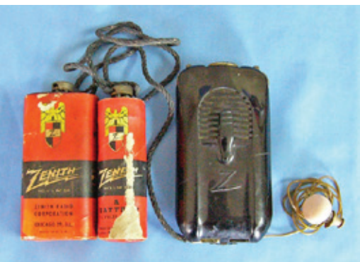
Figure 16. The Zenith Model A3A-B3A "Radionic" – a two-piece vacuum-tube hearing aid. The large "B" battery is on the left and the round "A" battery beside it (1944).
