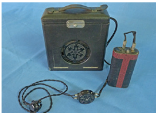
Figure 11. The Acousticon Model 28 carbon hearing aid – a lower-powered single carbon microphone hearing aid shown in its resonant case (1927).
