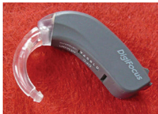
Figure 26. The Oticon Model DFC "DigiFocus Compact" BTE – one of the first completely digital BTE hearing aids made (1996).
