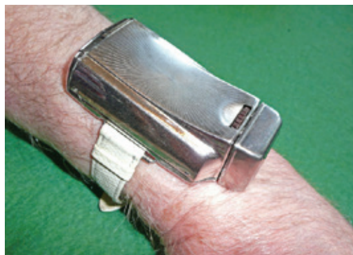
Figure 17. Acousticon's Model A-165 was the only wrist-worn vacuum-tube hearing aid ever made (1950).
