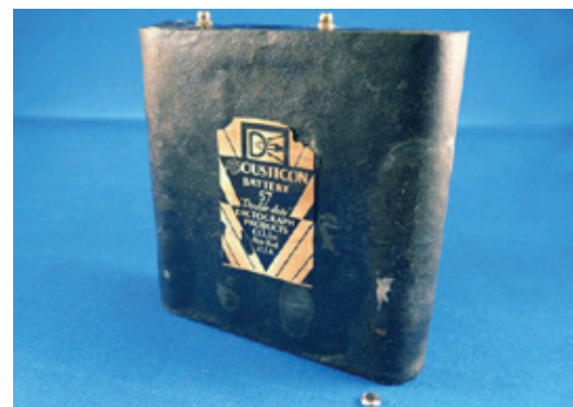
Figure 27. The Acousticon No. 57 hearing aid battery – one of the largest hearing aid batteries made contrasted with the tiny Panasonic No. 5 battery – the smallest hearing aid battery made.
