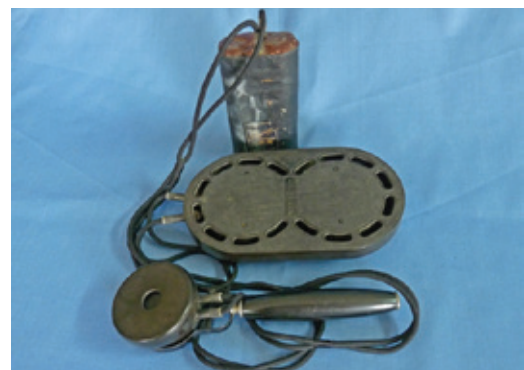
Figure 12. The Acousticon Model SRD was a medium-powered double carbon microphone hearing aid. You could wear the double-carbon microphone around your neck or clipped to your shirt-front (1910 – 1928).
