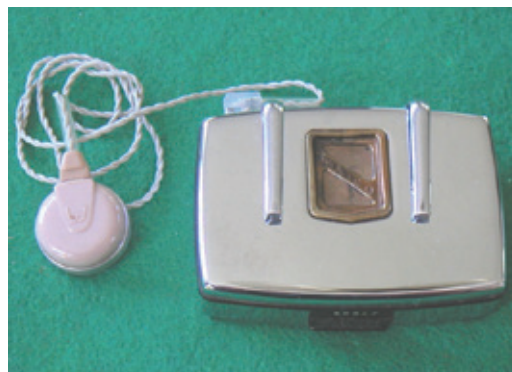
Figure 20. Maico's Model O "Transist-Ear" was the world's first all-transistor body hearing aid (January 1953).
