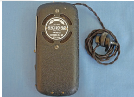
Figure 14. The “tiny” Electro-Ear Model 5 wearable carbon hearing aid had internal batteries (c. 1938).
