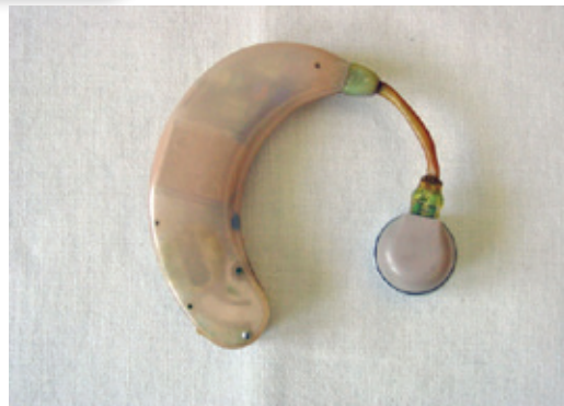
Figure 23. The humongous Zenith "Diplomat" BTE hearing aid – Zenith's first BTE hearing aid (June 1956).
