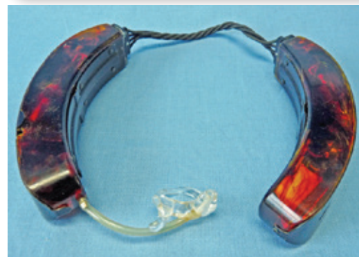
Figure 18. Acousticon's Model A-200 – a rare double-barrette vacuum-tube hearing aid for the ladies (1951).
