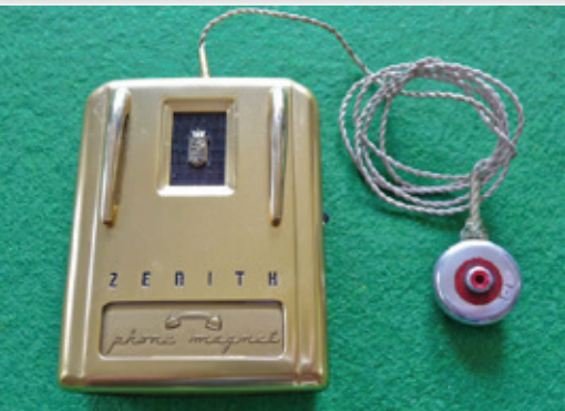
Figure 22. The Zenith "Royal T" was Zenith's first all-transistor hearing aid (Feb, 1953). It was the same size as the "Royal" vacuum-tube aid. Note that it had a t-coil built in – called a "phone magnet" in those days.
