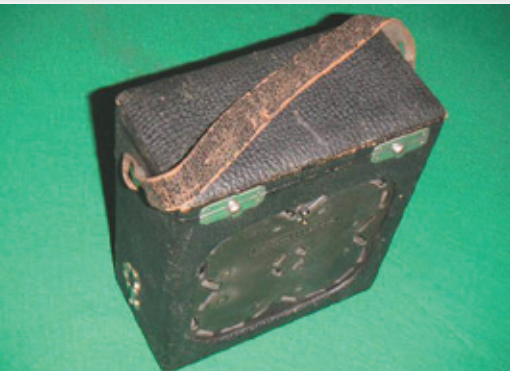
Figure 13. The high-powered (4 microphone) Acousticon Model RF carbon hearing aid had a six-step volume control on the left end of the case to reduce the volume if it was too loud (1910 – 1923).
