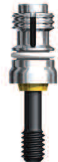
Figure 12. Expandable abutment: as the abutment-screw is tightened, the four “wings” of the abutment’s collar expand and engage the prosthesis thereby securing it to the implants.
