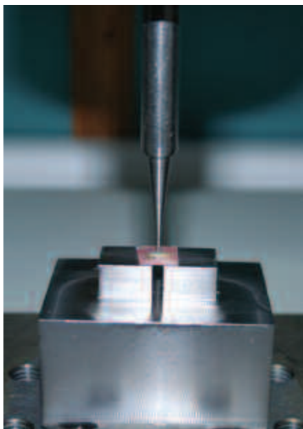
Figure 2. The post segments were loaded with a conical plunger for the push-out test.
