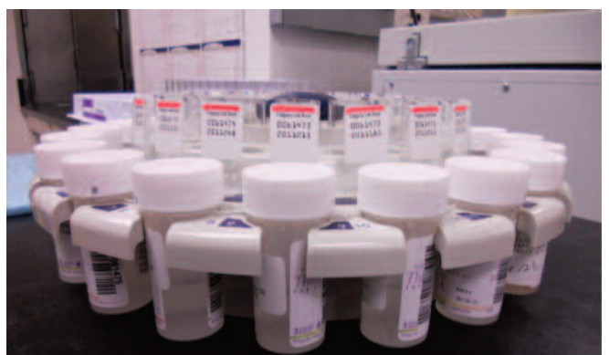
Figure 6. Carousel of specimens for processing by the T5000 processor.
