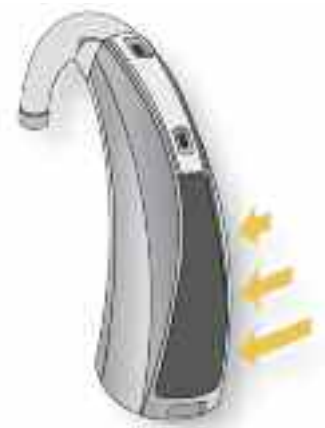
Figure 2B. An S Series hearing aid is shown. The arrows illustrate the tap motion that, by default, triggers a change in memory.
