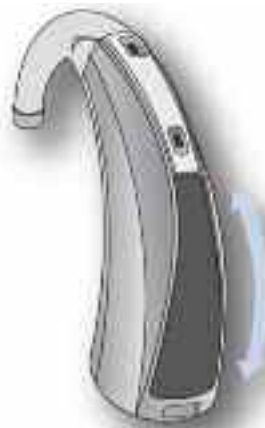
Figure 2A. An S Series hearing aid is shown. The arrows illustrate the sweep motion that, by default, triggers a change in volume.
