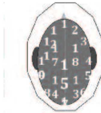
Figure 2. Illustration of the numbering chart used to locate the perceptual experience for the various signals. Listeners were asked have the experimenter adjust the relative left-right levels until the stimulus was perceived in a position as near as possible to number 15.
