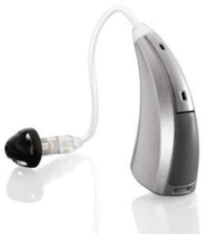
Figure 1. Starkey S series, non-occluding, receiver in the canal (RIC) hearing instrument.
