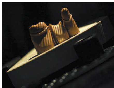
Figure 2. Projection of strip patterns on a model.
