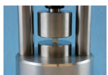
Figure 2. Disc specimen mounted in the testing device assembled for DTS testing.
