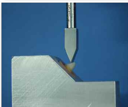
Figure 2. Specimens were loaded lingually at 135 degrees to the long axis with a compressive force.
