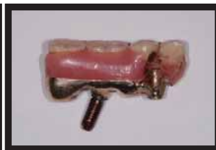
Figure 9 — fractured cantilever segment of full arch prostheses from Fig.8
