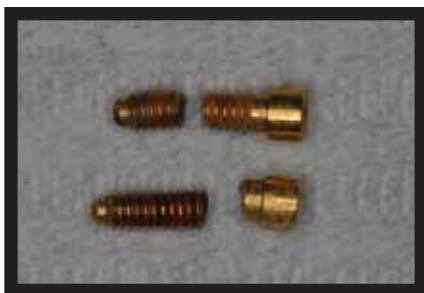
Figure 7 — retrieved fractured screws from Fig.6
