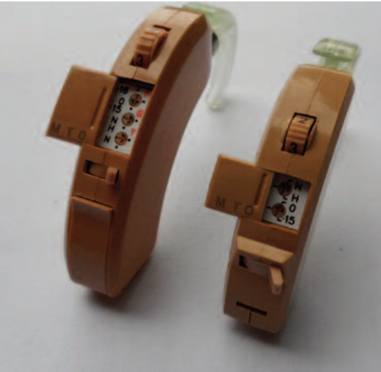
Figure 1. These are two Unitron BTEs of yesteryear. On the left is the UEI2, and on the right is the “mini” UM60. Aside from its large size and obligatory volume control, note the trimmers at the centre of each, which could be turned with a small screwdriver. These were “potentiometers;” turning them makes them work much like a dimmer switch for a dining room light. The left has 3 trimmers, for MPO (top), Gain (centre), and Tone (bone controls like these functioned much)
